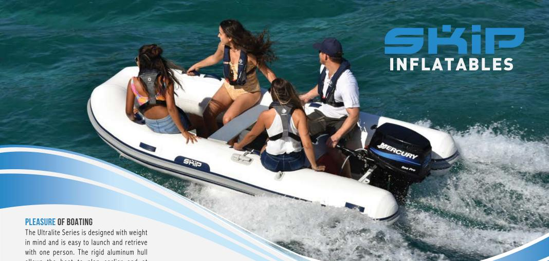
allows the boat to plan earlier and at lower speeds than soft bottom tenders. An increase in performance, fuel efficiency and the ability to plane with and increased payload are also very handy benefits of an aluminum rigid hull. Our boats are top quality and packed with features.
